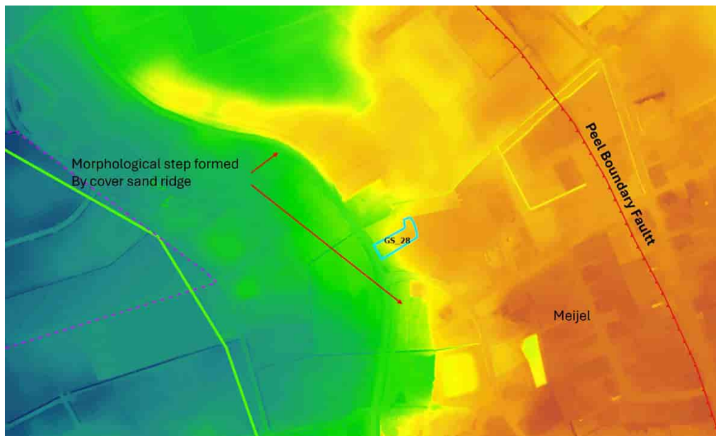
AHN image around GS_28 showing that the terrace step does not coincide with the Peel Boundary Fault but with the edge of a cover sand ridge
